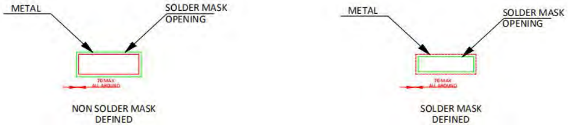
Figure 9.2 SOW8 Package Board Layout Example
